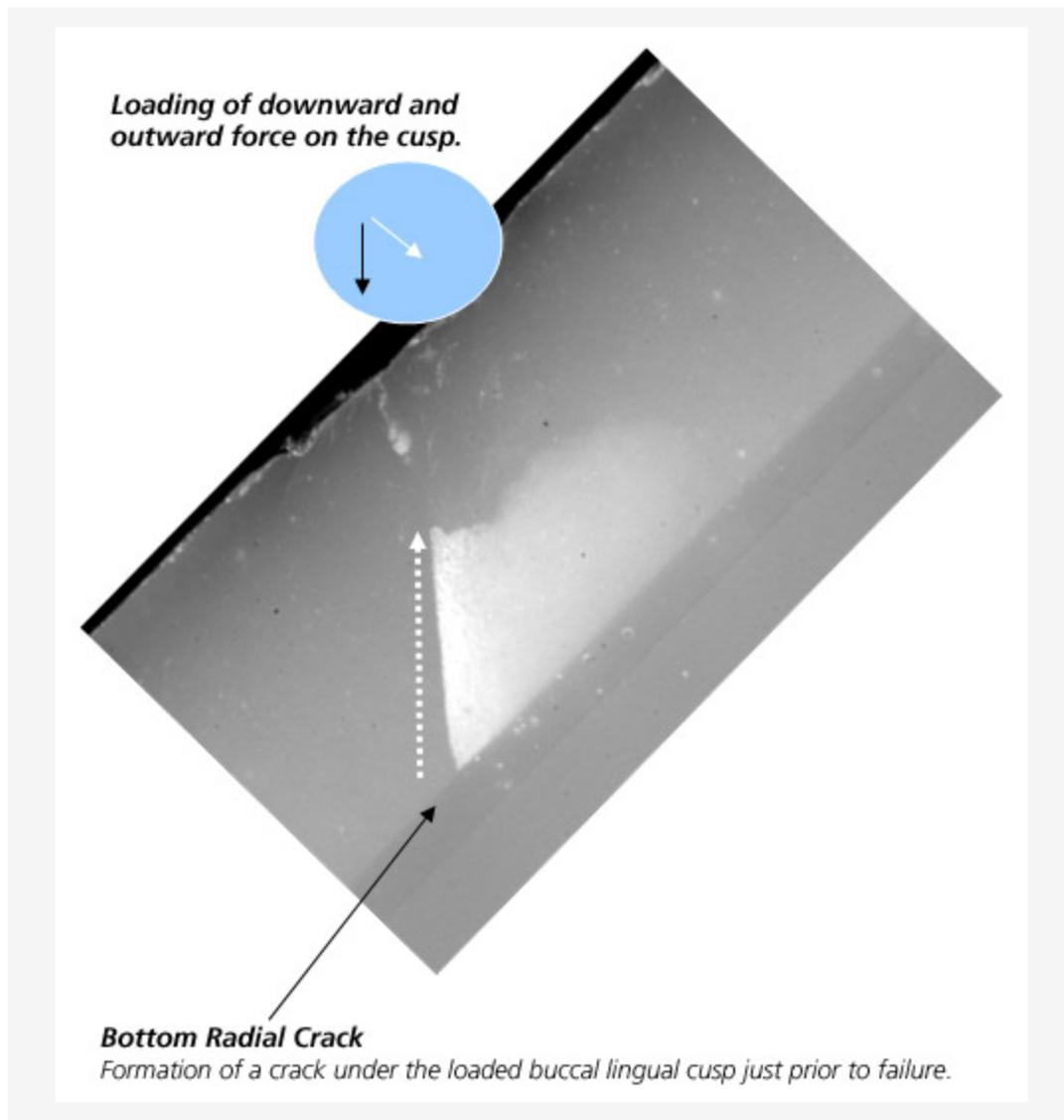
Test results showed that monolithic lithium disilicate outperformed veneered zirconia restorations. Through a 1,000N load and 1,000,000 cycles, none of the lithium disilicate crowns fractured. Only superficial damage in the form of wear facets similar those of natural teeth can be observed.
